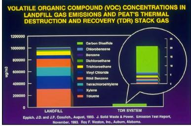
Comparison of Landfill Emissions vs. Plasma Pyrolysis
