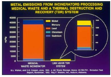
Comparison of Emissions—Incineration vs. Plasma Pyrolysis
